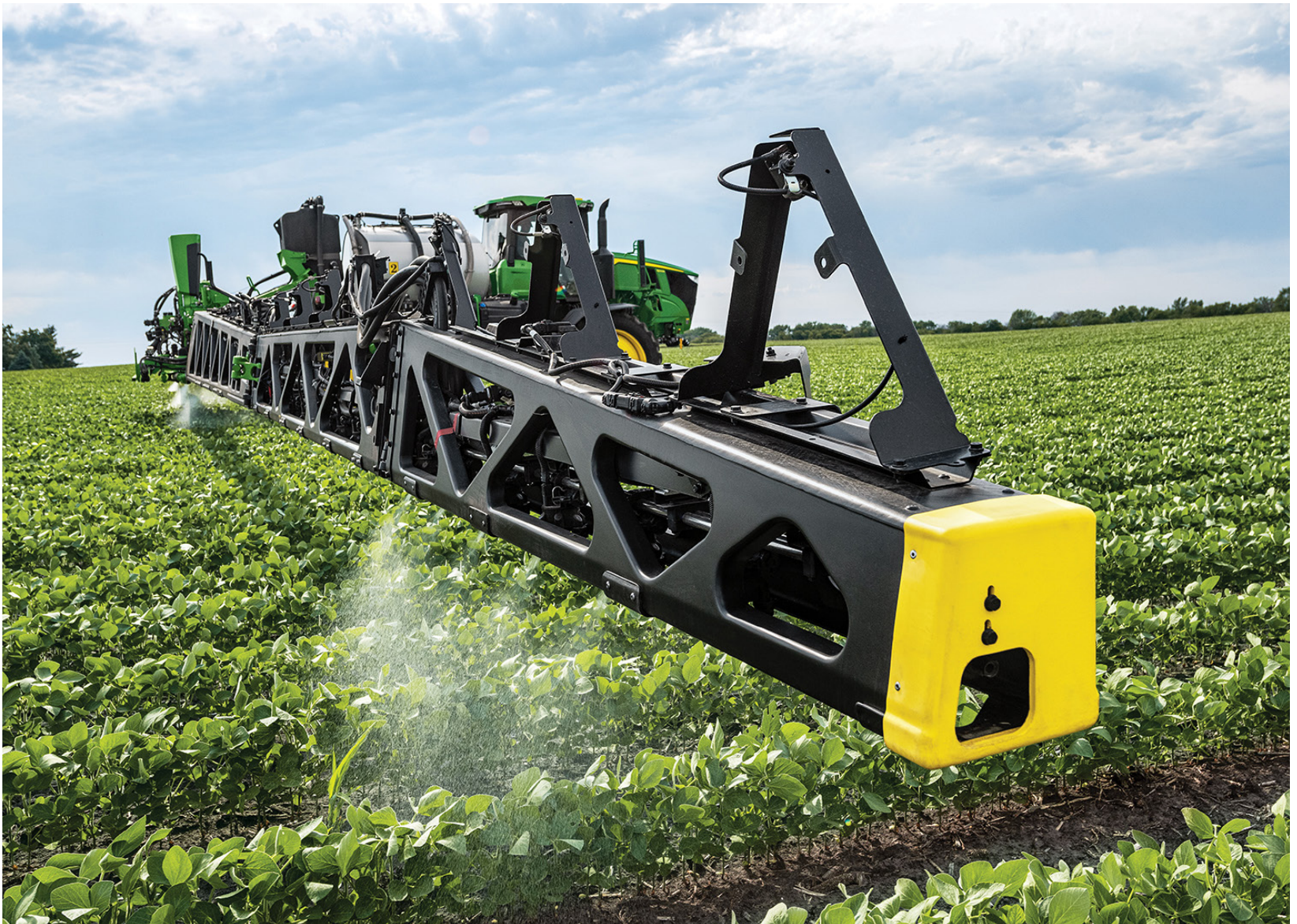
AI-enabled See & Spray™ technology allows farmers to identify and spray individual weeds, ensuring they apply herbicide only where needed. Photo credit: John Deere
