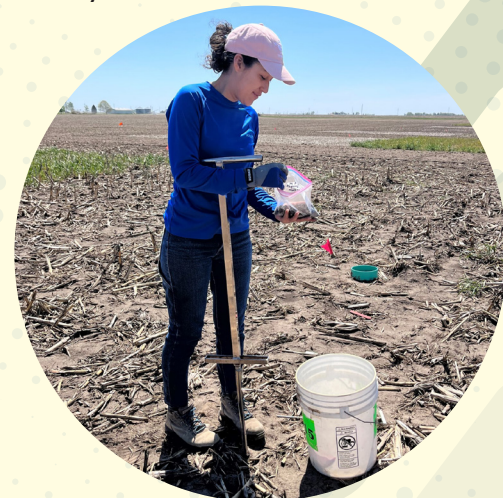
Field technician Guadalupe Gonzales collects surface soil samples (0-15 cm) in Monmouth in May 2023. Photo Credit: Heidi Allen Asensio
